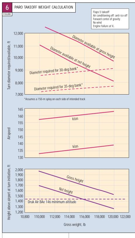
is solely a function of true airspeed and bank angle, and the turn diameter available at the corresponding net height.
