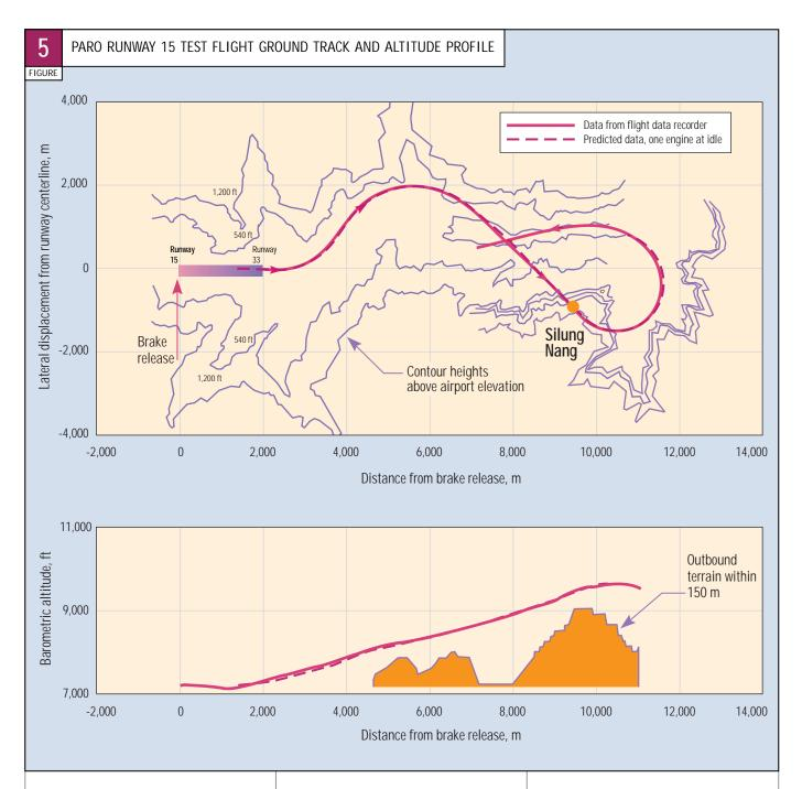
The calculated altitudes at the turnback initiation points for both flights were within 50 ft (15 m) on the conservative side of the predicted altitudes.
