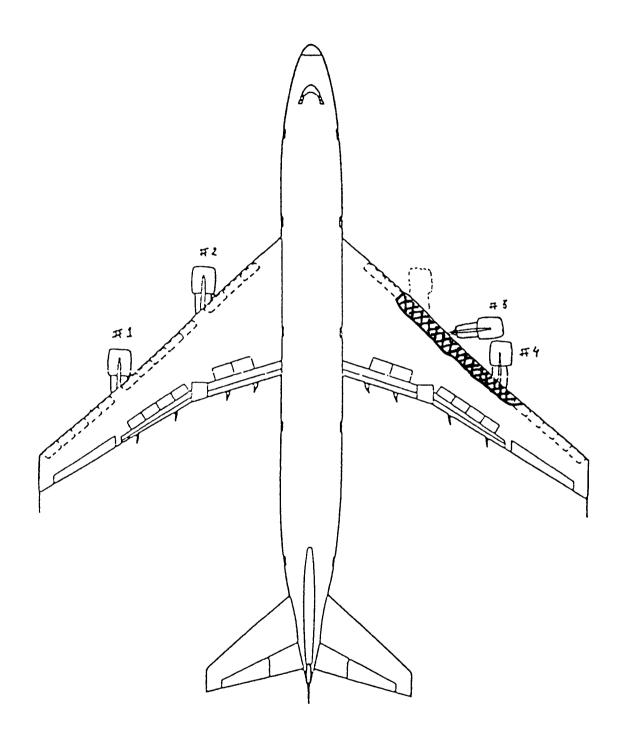
Figure 4. ESTIMATED DAMAGE TO RH WING LEADING EDGE
