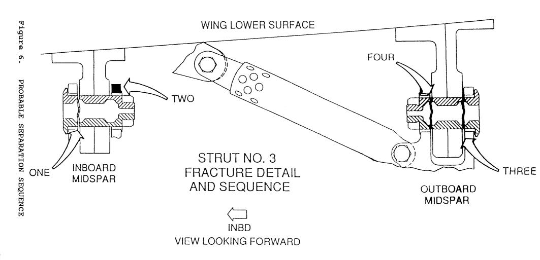
As there is no in service evidence that the El Al airplane experienced a static overload preceding the accident it is assumed that the inboard shear face of the fuse pin was initially fatigued and then failed under normal flight conditions. Based on this assumption separation scenario 2 was further develo-
