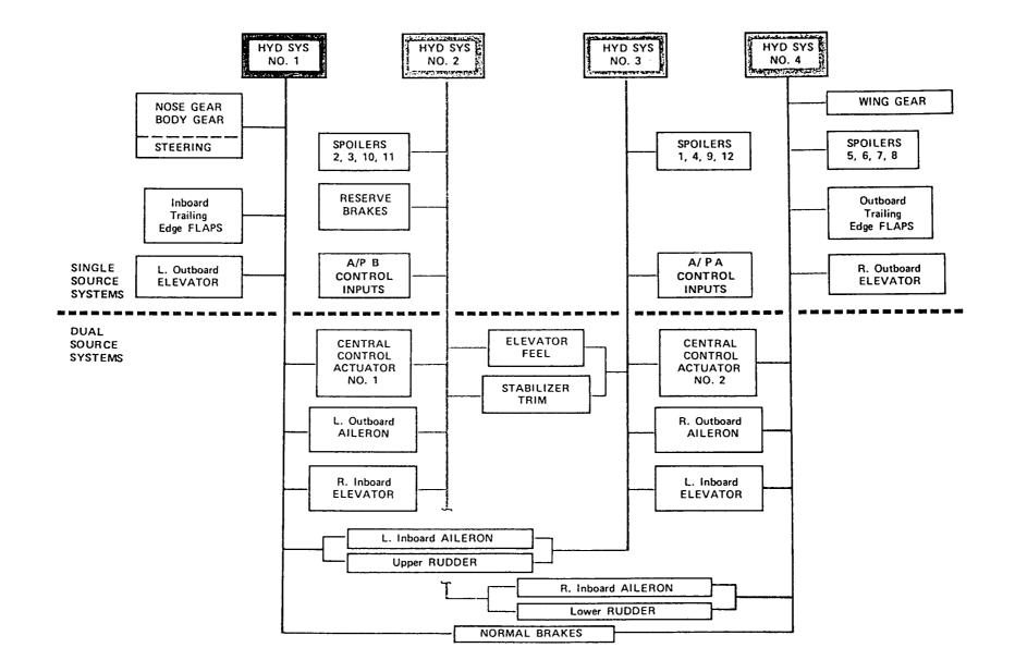
Figure 2. HYDRAULIC POWER SYSTEM
