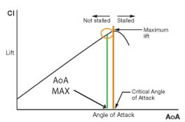
Figure 2 In ALTERNATE and DIFECT LAW, the aural Stall Warning is set at a value lower than AoA STALL
