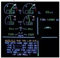
Figure 34: The ECAM messages after RTLU 1 and 2 fault
