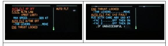
Figure 33: The page 1 and 2 of the ECAM messages after CBs of FAC 1 and 2 being reset
