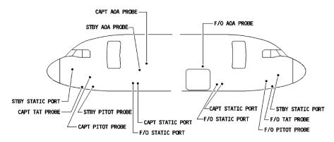
**Figure 12: The Pitot Static Configuration**
