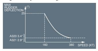
If both FACs lose the rudder travel limitation function, the value of the rudder deflection limit is locked at the time of the second failure.
