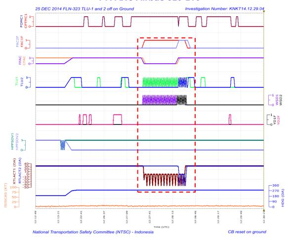
Figure 24: The FDR parameters of FAC fault followed by CB reset on the ground at 25 December 2014
