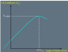
Lift Coefficient versus Angle of Attack.
