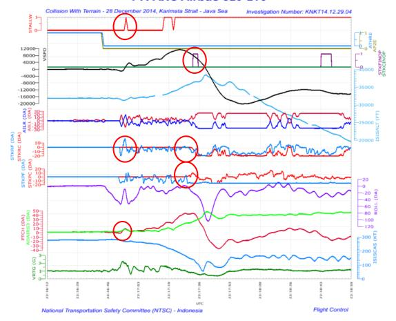
Figure 22: Pilots inputs on side stick
