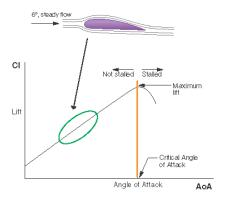
When the AoA reaches the value of the maximum Cl, the airflow starts to separate.
