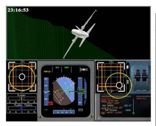
Figure 25: Aircraft rolled  $54^{\circ}$  to the left
