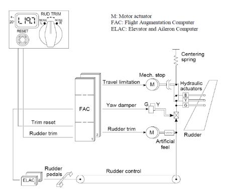
Figure 8: Rudder command architecture
