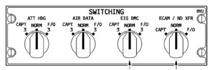
Figure 11: Switching panel on pedestal
