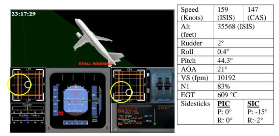
Figure 27: The aircraft attitude at the highest pitch angle
