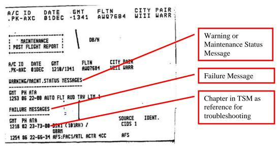
Figure 6: Typical Printed Post Flight Report (PFR)
