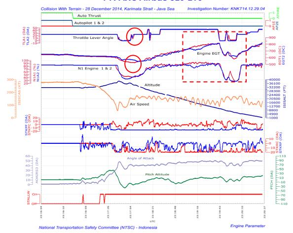
Figure 23: Thrust levers and side-sticks movement
