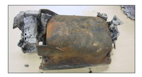
Figure 2: PK-GZC flight data recorder as received at the ATSB on 9 March 2007
