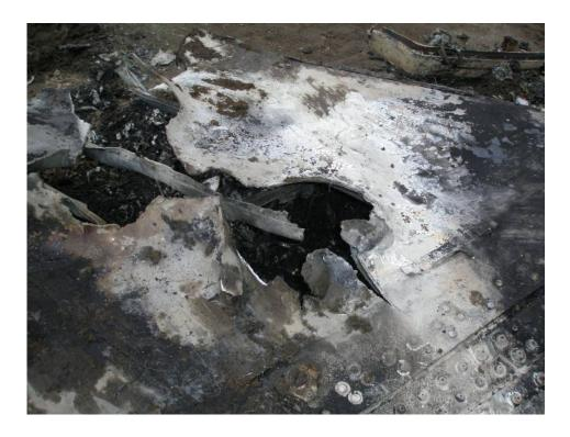
Figure 21: Close-up view of fuel burn explosion damage to right wing
