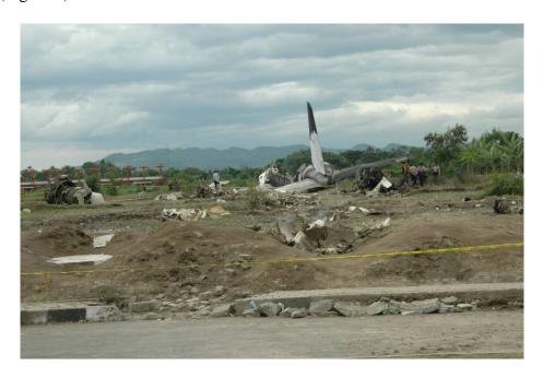
Figure 6: Left engine impact on road and gutter
