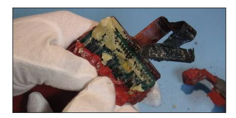
Figure 4: SSFDR memory board connector pins and damaged flex cable
