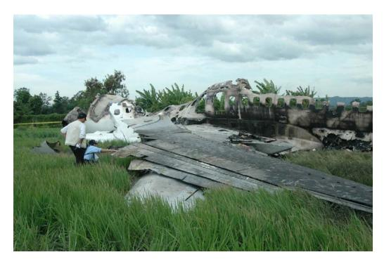
Figure 17: Severed right wing on the left wing
