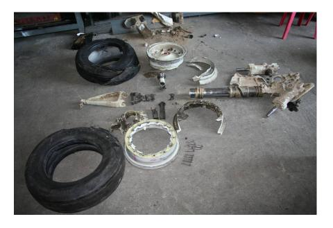
Figure 5: Nose landing gear wreckage layout
