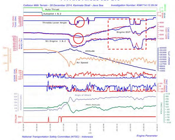
Figure 23: Thrust levers and side-sticks movement
