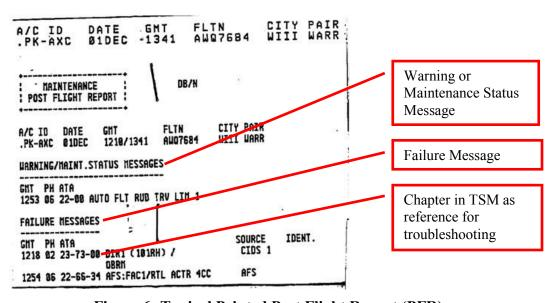
Figure 6: Typical Printed Post Flight Report (PFR)
