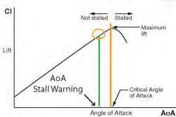
The EFCS adjusts the AoA MAX limitation to account for the reduction of the AoA STALL with increasing Mach number.
