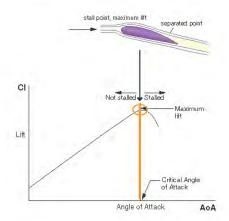
Beyond this point, the lift decreases as the flow is separated from the wing profile. The wing is stalled.
