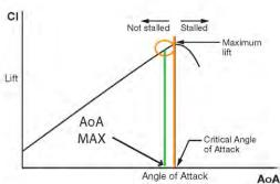
Figure 2 In ALTERNATE and DIRECT LAW, the aural Stall Warning is set at a value lower than AoA STALL
