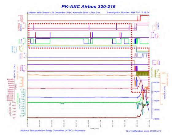
Figure 20: RTLU problems and pilot actions
