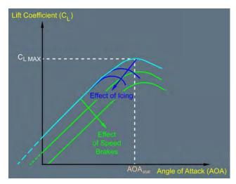
On the contrary, speed brake extension and ice accretion reduce the maximum lift coefficient.
