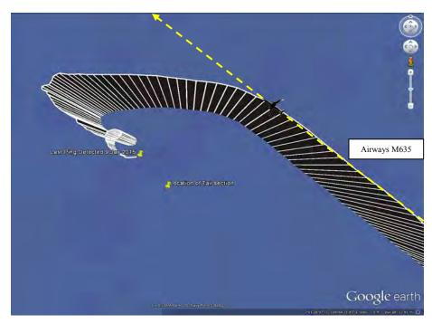
Figure 19: Flight path based on FDR data superimposed to the Google Earth Detail information of the FDR is shown on the following graphs.
