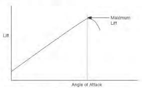
For a given configuration, a given speed and a given altitude, the lift is only linked to the AoA.
