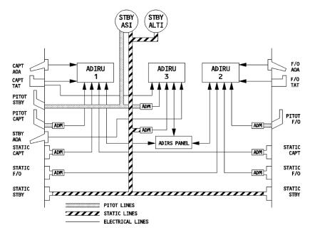
Figure 13: line probes schematic
