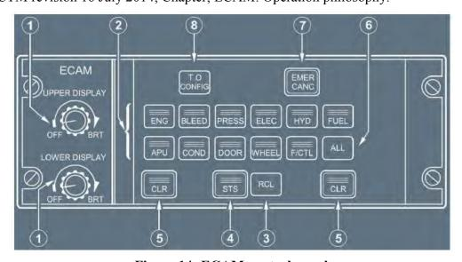
Figure 14: ECAM control panel
