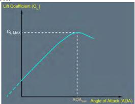
Lift Coefficient versus Angle of Attack.
