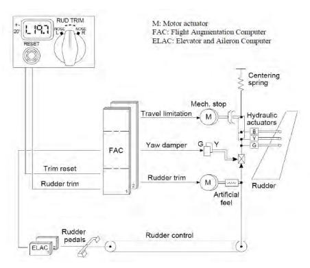
Figure 8: Rudder command architecture
