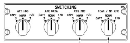
Figure 11: Switching panel on pedestal
