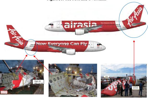
Figure 32: Pictures of identified parts and its original position
