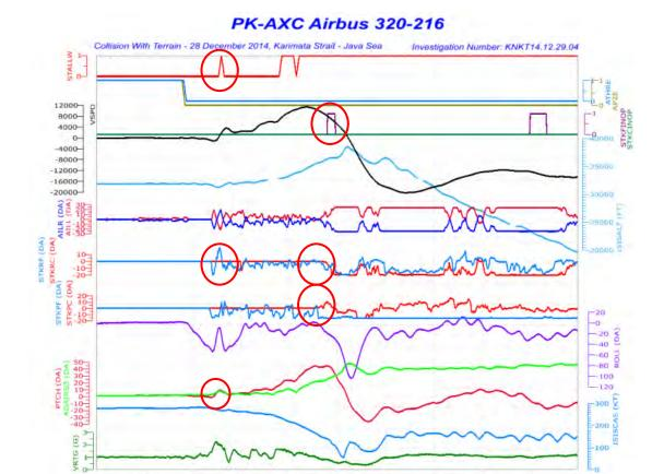
Figure 22: Pilots inputs on side stick
