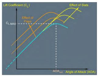
Influence of Slats and Flaps on Lift Coefficient versus Angle of Attack, Slats and Flaps have a different impact on the Lift coefficient obtained for a given AOA. Both Slats and Flaps create an increase in the maximum lift coefficient. Influence of Speed Brakes and Icing on Lift Coefficient versus Angle of Attack.
