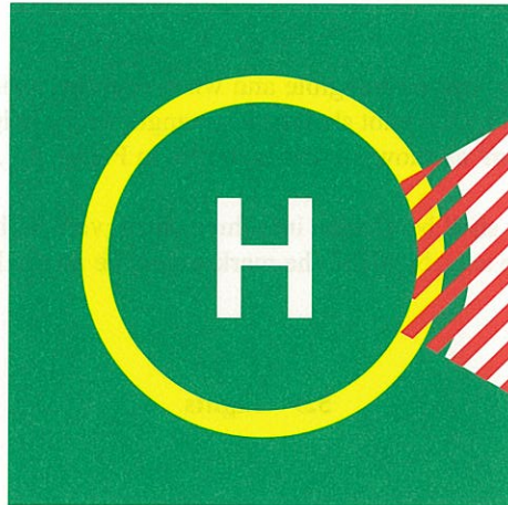
Figure 5-5. Helideck prohibited landing sector marking
